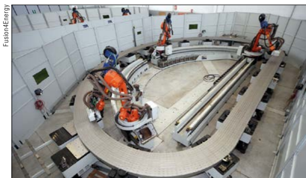
Laser welding of the toroidal field coil taking place.
