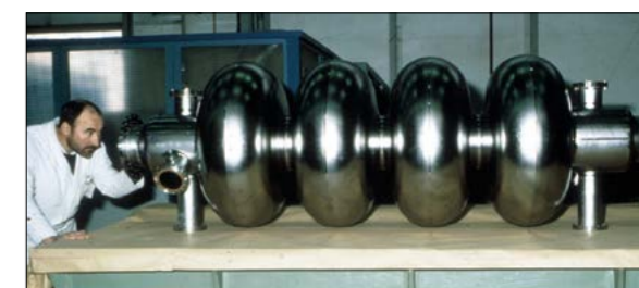
The copper cavities used to accelerate particles in LEP (above). Replacement superconducting RF cavities installed in the LEP tunnel (above right) and their niobium accelerating structures (bottom right) allowed the collider's energy to be doubled in the late 1990s, beyond the pair-production threshold for W bosons.
