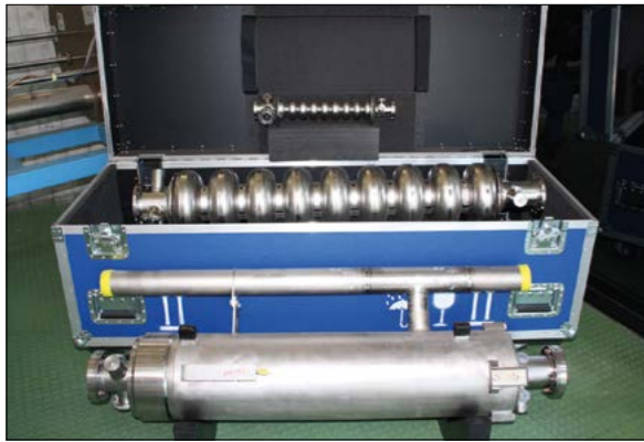
The European XFEL cavity family: a 1.3 GHz naked (in case) and dressed (bottom), and the smaller 3rd harmonic, 3.9 GHz cavity (top) used to linearise the longitudinal phase space.
