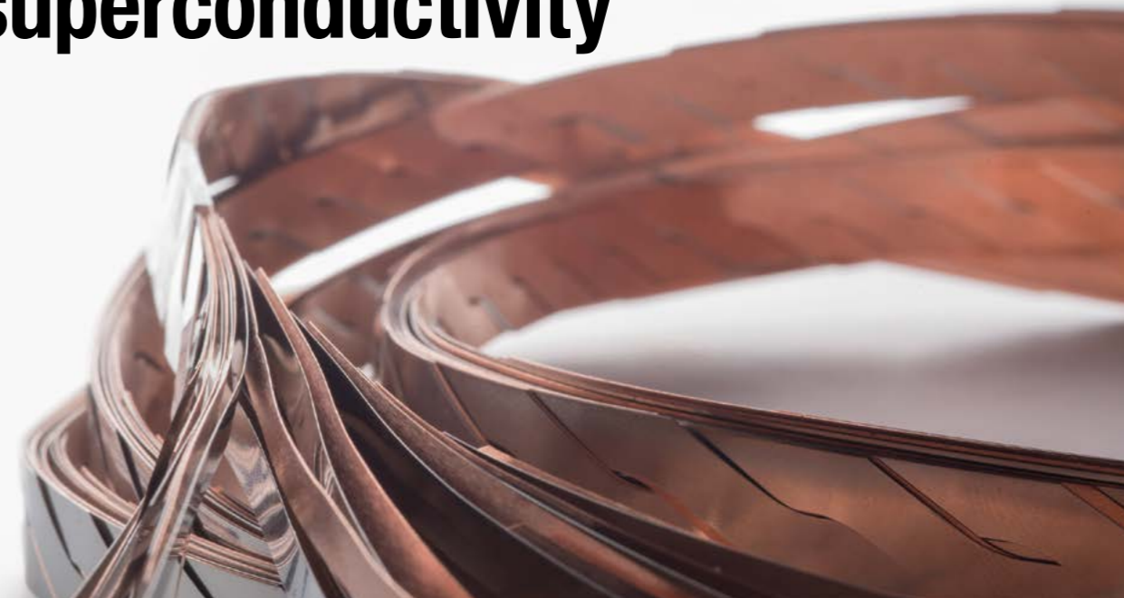
Prototype "Roebel" cable based on the high-temperature superconductor REBCO (rare-earth barium-copper oxide) is being used to wind a demonstration accelerator dipole at CERN as part of the EuCARD-2 project. (Image credit: H Barnard/CERN.)
