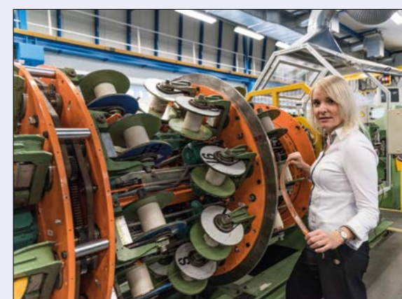
Assembling niobium-tin Rutherford cable at CERN, with Amalia Ballarino, head of the superconductors section in CERN's technology department.
