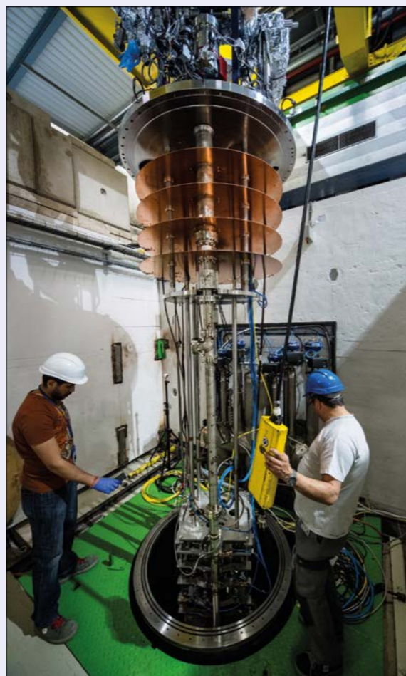
The double quarter-wave crab cavity assembled on the RF test stand for cold testing in a vertical cryostat at CERN's SM18 facility.
