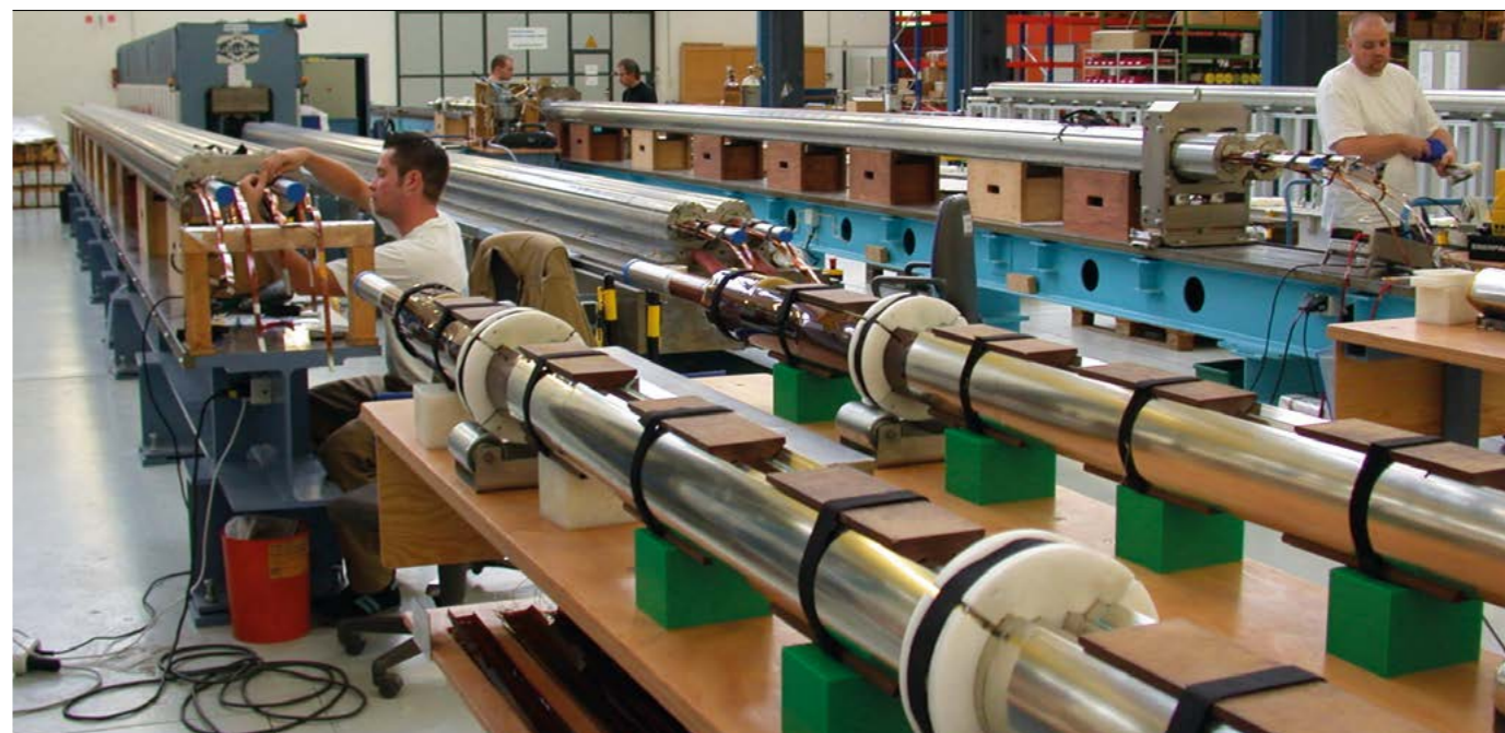
Assembly of the LHC's superconducting dipoles in 2003 at the German company Babcock-Noell, one of the three European industrial centres of production for the LHC's 1232 main dipole magnets. (Image credit: CERN.)
