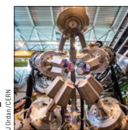
The Miniball germanium array, which uses beams from the upgraded HIE-ISOLDE facility.
