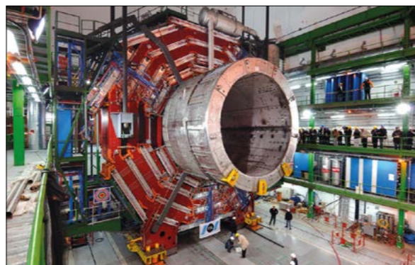
(Above) The far-from-compact CMS solenoid in position in the detector. (Left) One of the ATLAS end-cap toroids arriving at the ATLAS surface building in May 2007.
