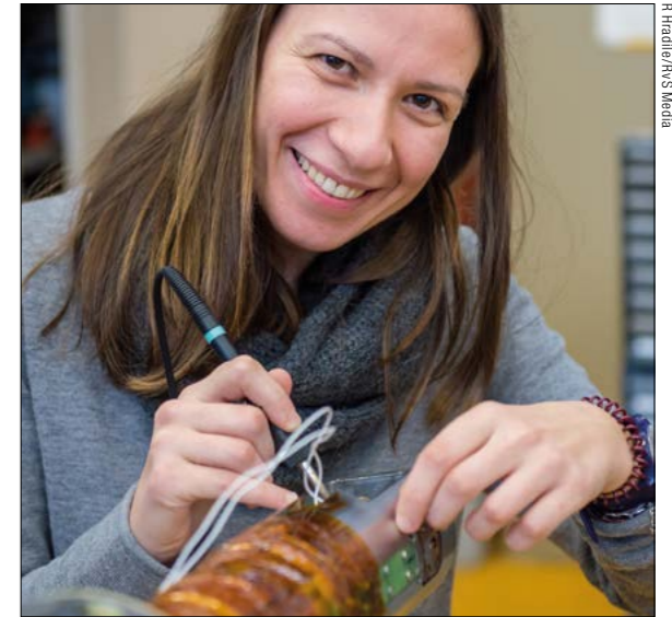
CERN fellow Konstantina Konstantopoulou working on a new generation of MgB 2 superconductors for future colliders.
